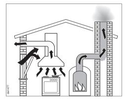
Ventilation can be maintained by air inlets which must not be blocked, in windows, doors and outside wall vents, or by other technical measures, such as ensuring that the cooker hood can only be switched on when the heating appliance is switched off or vice versa. A ventilation brick alone is not generally sufficient to ensure safe ventilation.
